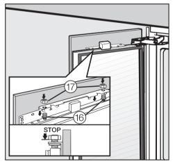
Open the appliance door and hang the furniture front on its frame onto the threaded bolts, as shown <sup>(6)</sup>.
